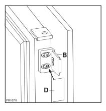
If the appliance is fixed to the side of the kitchen unit, simply slacken the screws in the fixing brackets (E), move the brackets as shown in the figure and re-tighten the screws.
